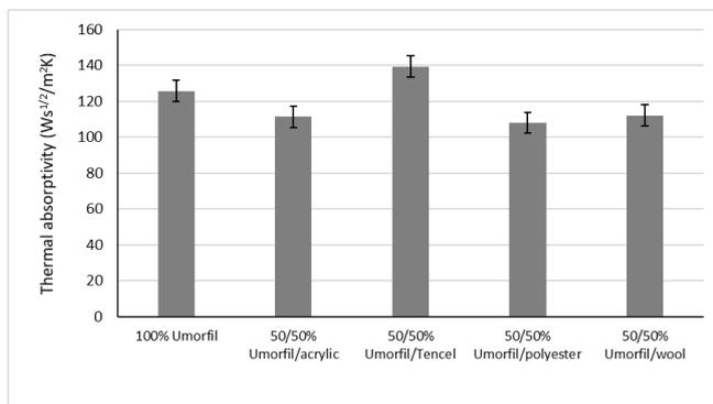
Figure 6. Thermal absorptivity results
