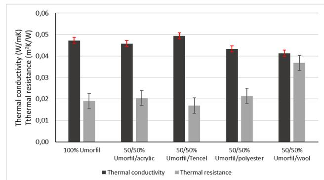
Figure 5. Thermal conductivity and thermal resistance results
