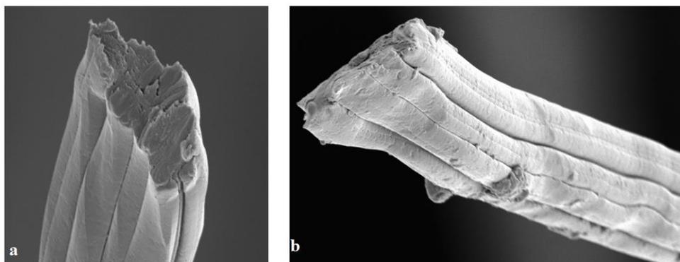
Figure 2. Cross-sectional (a) and longitudinal (b) view of the Umorfil® fibres
